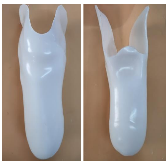
Figure 1: PTB-SC Socket Design (Anterior and Posterior View)
